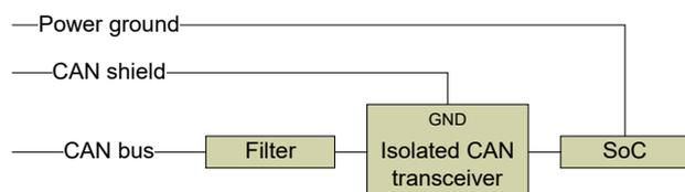
Figure 15: Isolated CAN port internal block diagram
