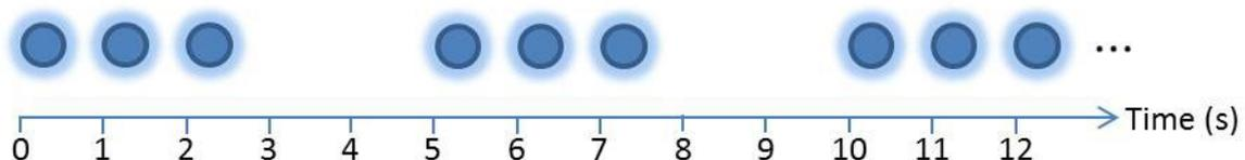
Figure 13: Example of the blinking pattern for error code 3
