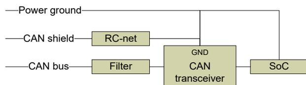
Figure 14: Non-isolated CAN port internal block diagram
